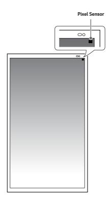
• Pixel Sensor: Measures the RGB of pixels in that area.
